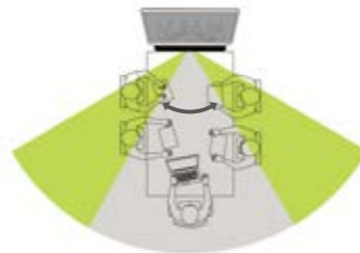
Ultra-wide angle camera with 120° field of view
